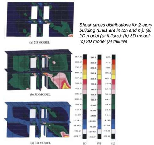
A combination of a distributed shear-wall mechanism and a story mechanism lead to the collapse stage accompanying the inelastic deformation. The overall system behavior was completely controlled by the symmetrically distributed shear walls. The 5-story case provided enhanced deformation capacity
