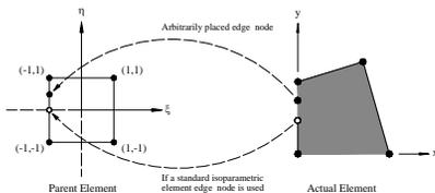
The capability of moving any of the element's edge nodes to any location along an edge allows these edge nodes to be placed in a proper position such that, they can serve as end nodes for the cover of the main discrete reinforcement. This provides a robust stiffness contribution coming from the main reinforcement.
