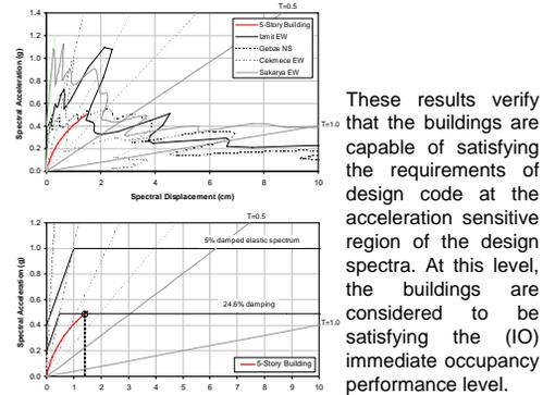
These results verify that the buildings are capable of satisfying the requirements of design code at the acceleration sensitive region of the design spectra. At this level, the buildings are considered to be satisfying the (IO) immediate occupancy performance level.
