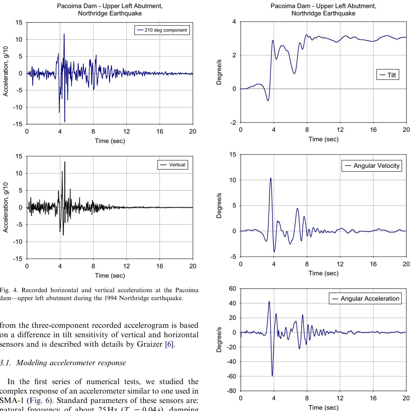
Fig. 4. Recorded horizontal and vertical accelerations at the Pacoima dam—upper left abutment during the 1994 Northridge earthquake.
