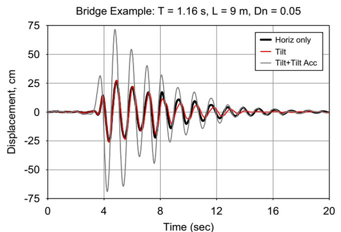
Fig. 12. Coupled effects of tilt and angular acceleration on the response.
