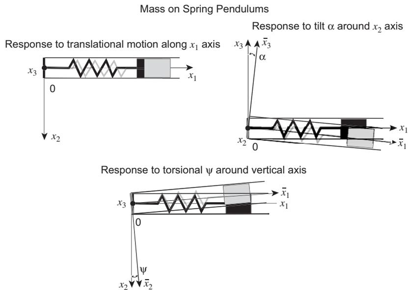
Fig. 2. Mass-on-spring pendulum and its response to complex ground motion (note:  $x_1$  and  $x_2$  lie in horizontal plane).
