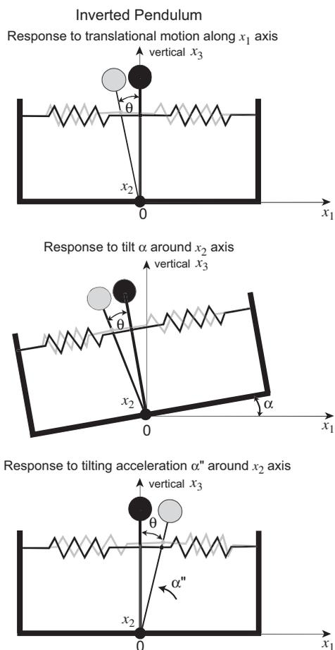
Fig. 3. Inverted (astatic) pendulum and its response to complex ground motion (note:  $x_1$  and  $x_2$  lie in horizontal plane).
