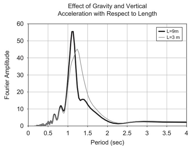
Fig. 11. Effects of pendulum length on translational response (top-panel) and Fourier amplitude spectrum (bottom-panel).
