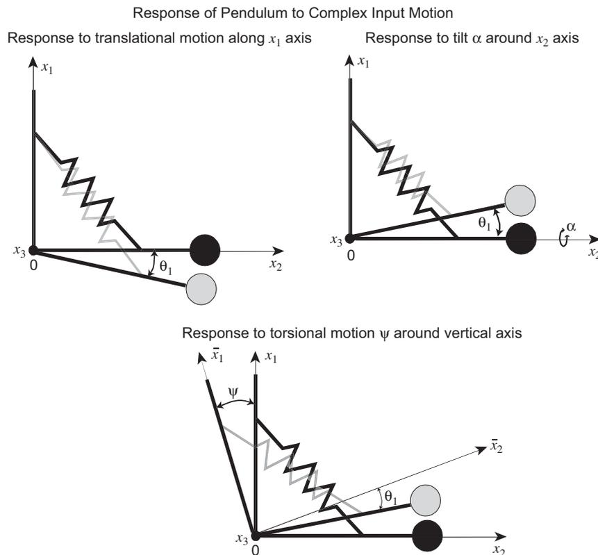
Fig. 1. Mass-on-rod pendulum and its response to complex ground motion (note:  $x_1$  and  $x_2$  lie in horizontal plane).
