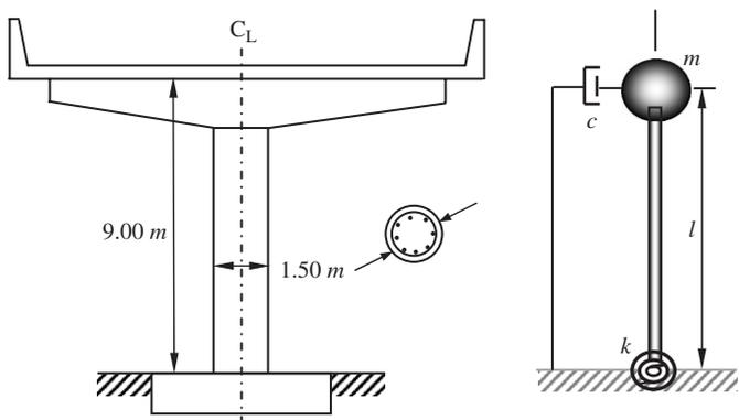
Fig. 8. Single column of a bridge bent and its idealized lumped-mass pendulum system.
