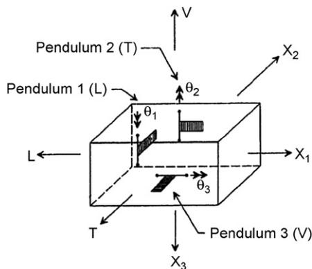
Fig. 6. Schematic representation of three transducers in an accelerograph. The coordinate axes  $X_1$ ,  $X_2$  and  $X_3$  serve to describe the motion of the  $L$ ,  $T$  and  $V$  transducers, respectively. Angles  $\theta_1$ ,  $\theta_2$  and  $\theta_3$  describe the deflection of the transducer pendulums (modified from Trifunac and Todorovska [17]).
