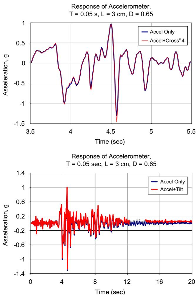
Fig. 7. Response of an accelerometer to cross-axis acceleration (top-panel) and tilt (bottom-panel).
