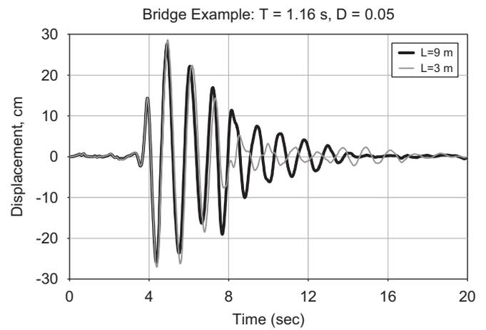
Fig. 10. Effects of polarity of vertical ground motion on translational response.
