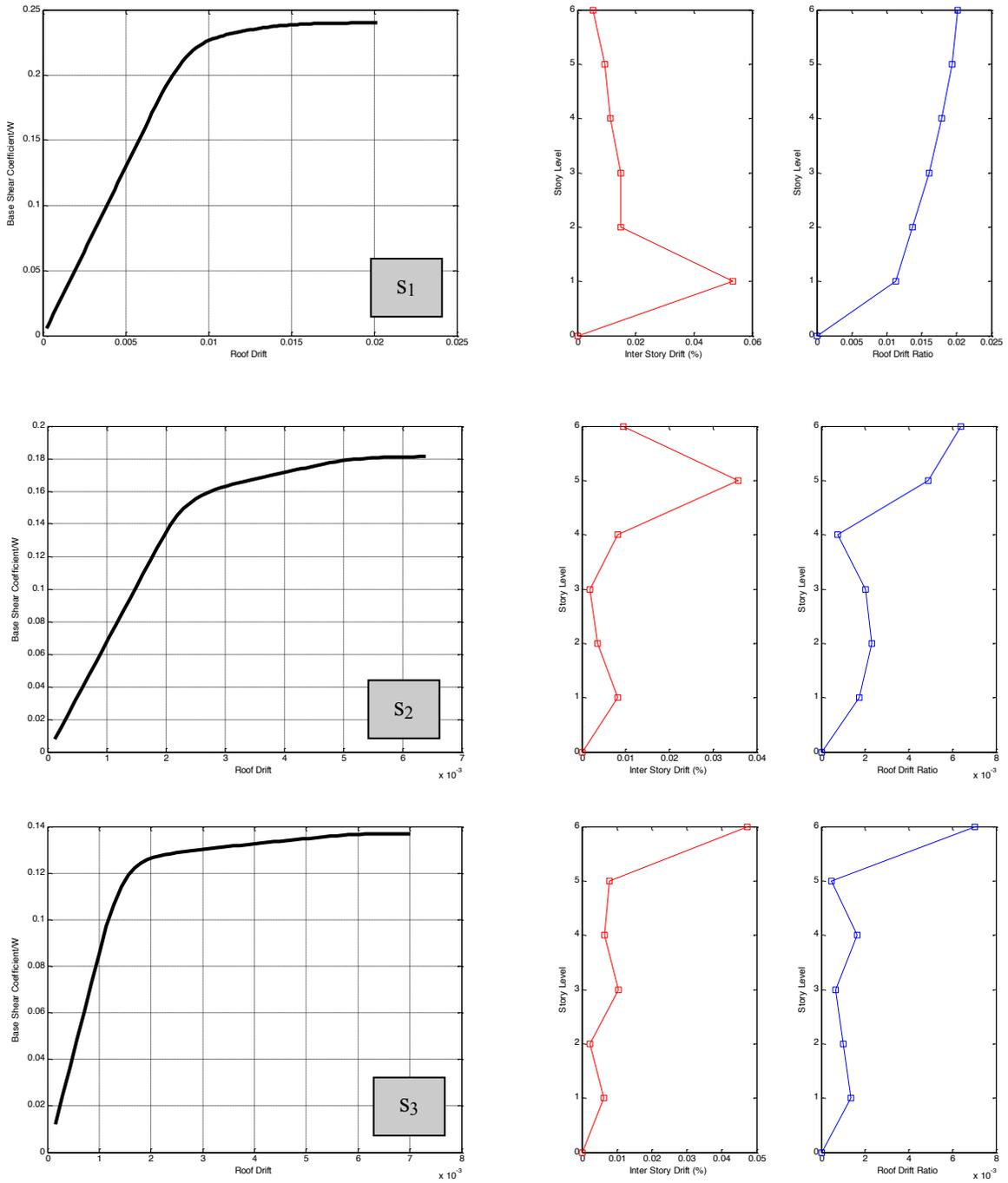
**Figure 7.** Capacity curve and interstory and roof drift profiles for six-story building based on separate pushover analyses using invariant load distribution of (a) s1, (b) s2 and (c) s3. Target displacement is 2 percent of roof drift for the first mode and 0.6 percent for the second and third modes.
