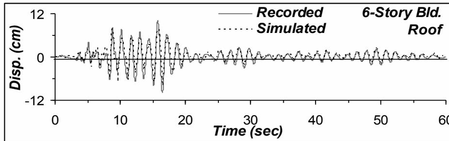
**Figure 4.** OpenSEES model validation (recorded and computed response at mid and roof levels).
