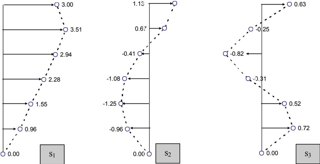
**Figure 6.** Height-wise distributions ( $s_n$ ) of invariant modal load vectors ( $s_n = mf$ ).
